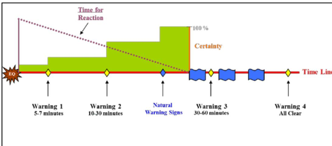
Figure 41: Estimated time from a local tsunami occurring until information is received with confirmation of the tsunami, and the limited reaction time (Source: GTZ IS-GITEWS)
